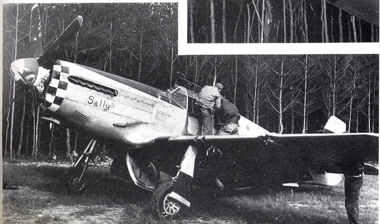
Right & below: P-51B, 'Sally' of the 339th Fighter Group safely back at its home base after flying through cables during a low level strafing run over France. Note cables dangling from spinner. (photos Ray E. Bowers).
