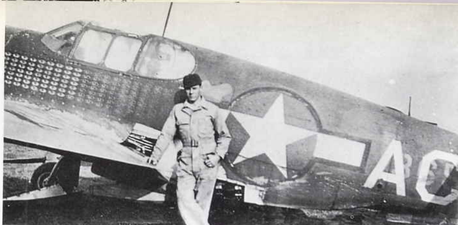
Left: P-51's of the 111th Tac Recon Squadron, 64th Fighter Wing, 12th Air Force, Sicily/Italy 1943. Note Recon missions indicated with eyes under cockpit. All aircraft modified for reconnaissance duties with camera behind cockpit.
