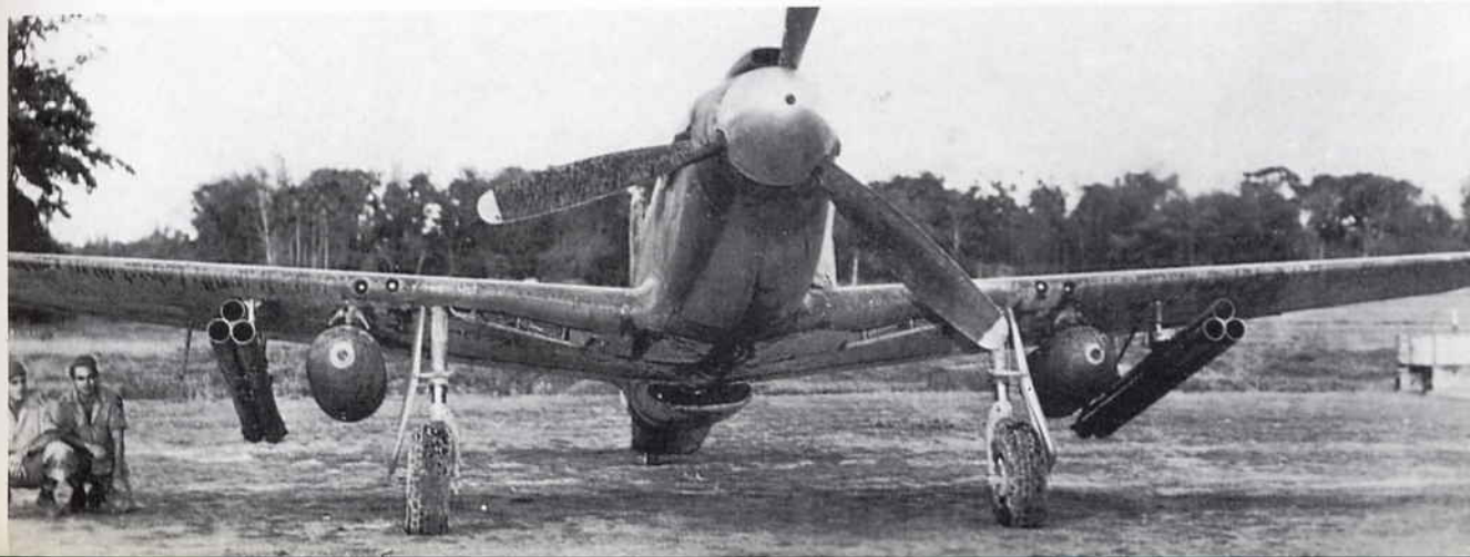
Below: Mustang bombed up and armed with Bazooka tubes on an Indian airfield. (USAF).
