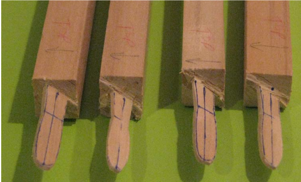
Figure 7 Propeller Blade Outlines Carved
