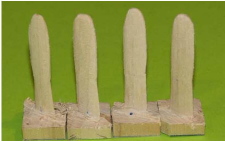
Figure 8 Propeller Blades Shaped & Profiled
