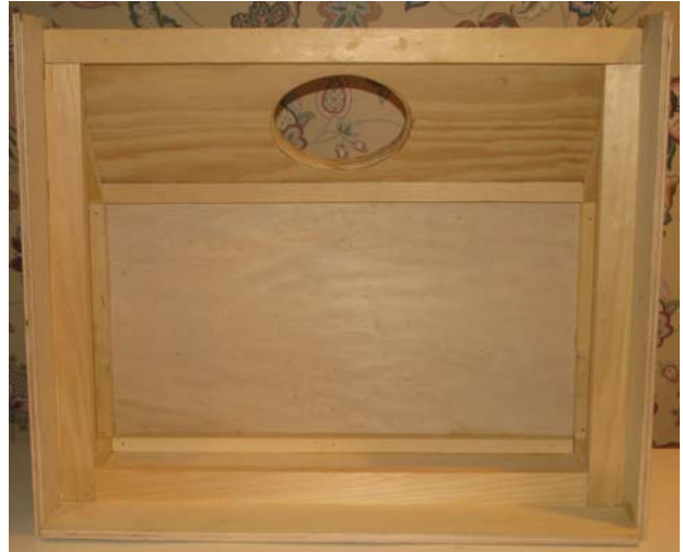
Figure 3 Sloped Back and Plenum Frame
