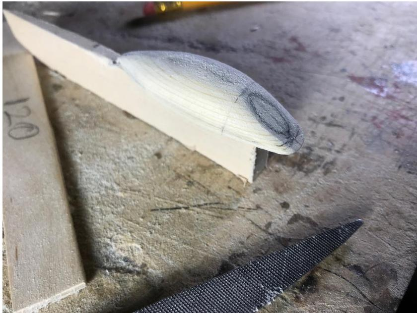
Note 1. Paint stir sticks available for free at most hardware/paint stores make excellent sanding tool. Application of a different sandpaper grit to each side doubles its value.
